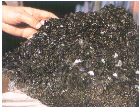
Figure 4. A cluster of black carborundum platelets (synthetic moissanite) produced by the Acheson process 2 for abrasives use.
