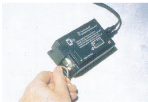
Figure 9. The Colourless Moissanite/Diamond Tester Model 590 of Charles and Colvard, designed to distinguish between diamond and synthetic moissanite only after a stone is given a 'diamond' reaction by a thermal probe. Photo by Maha DeMaggio, courtesy of GIA.
